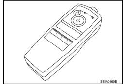
5. Register the IDs in order from FR LH, FR RH, RR RH or RR LH. When ID registration of each wheel has been completed, a buzzer sounds and hazard warning lamp blinks.
